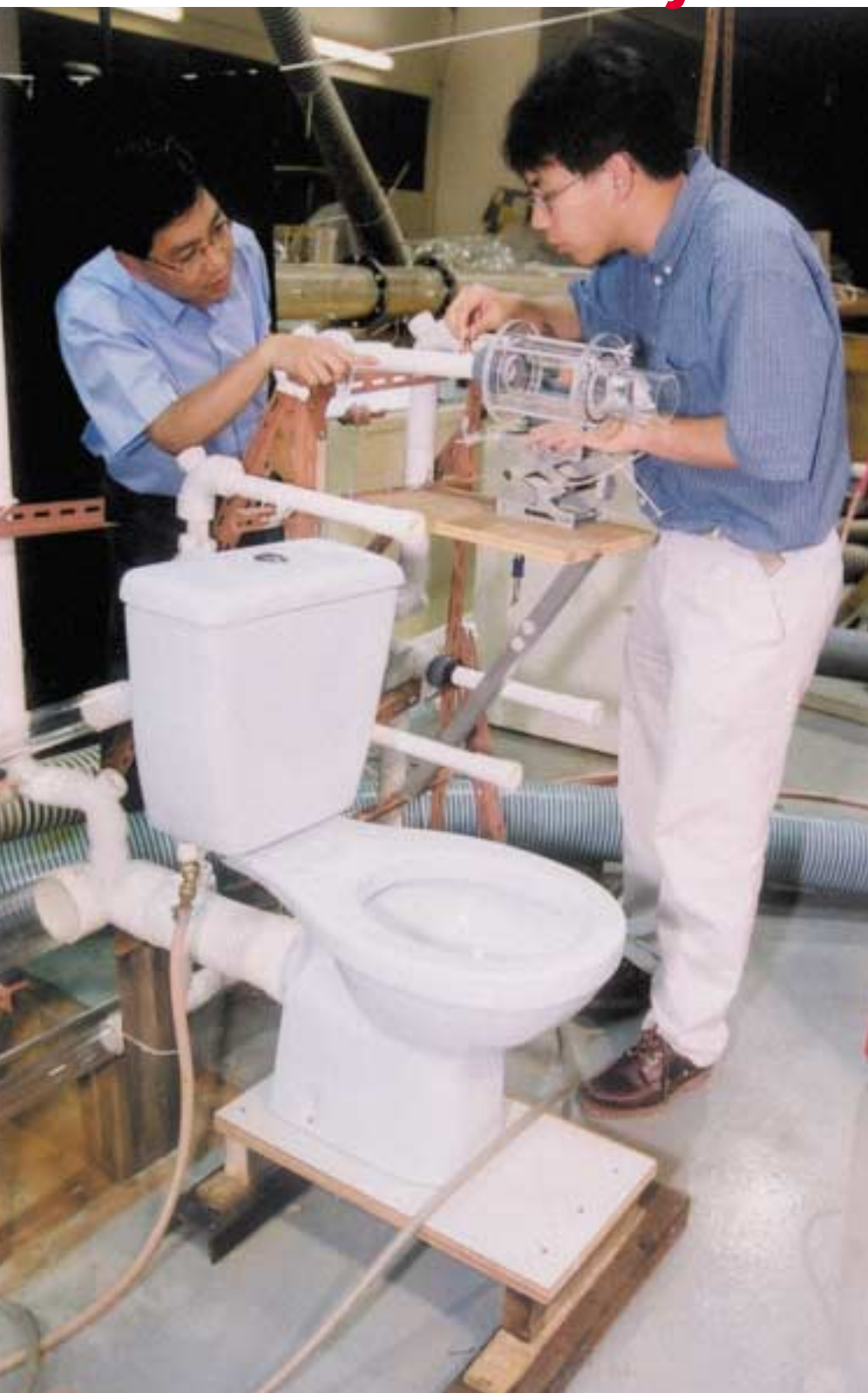
BELOW: Engineers Dennis Y C Leung (梁耀彰) and Andy Chan (陳德儀) investigated the Amoy Gardens outbreak by modeling the buildings' toilets and pipes.
